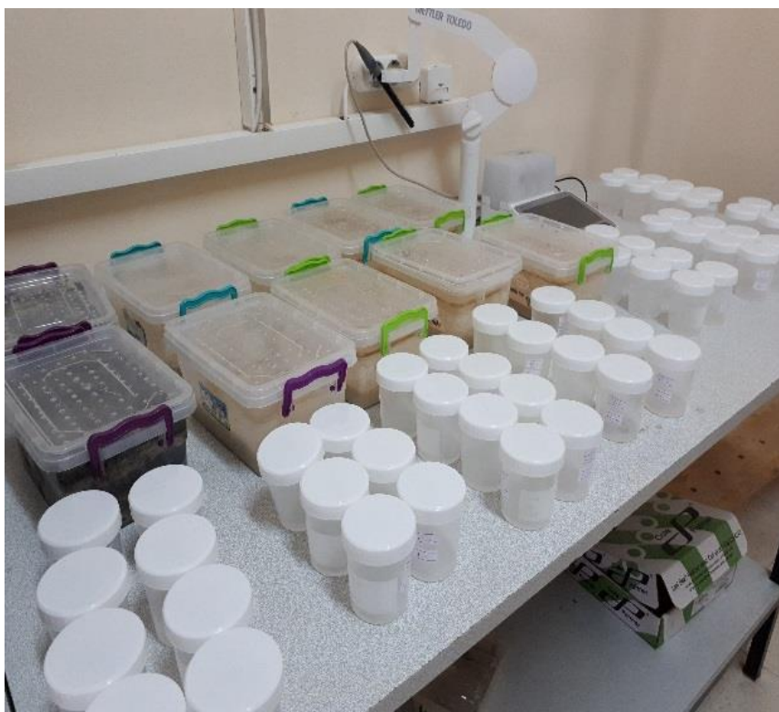
Fig. 2. Static tests conducted in plastic containers
