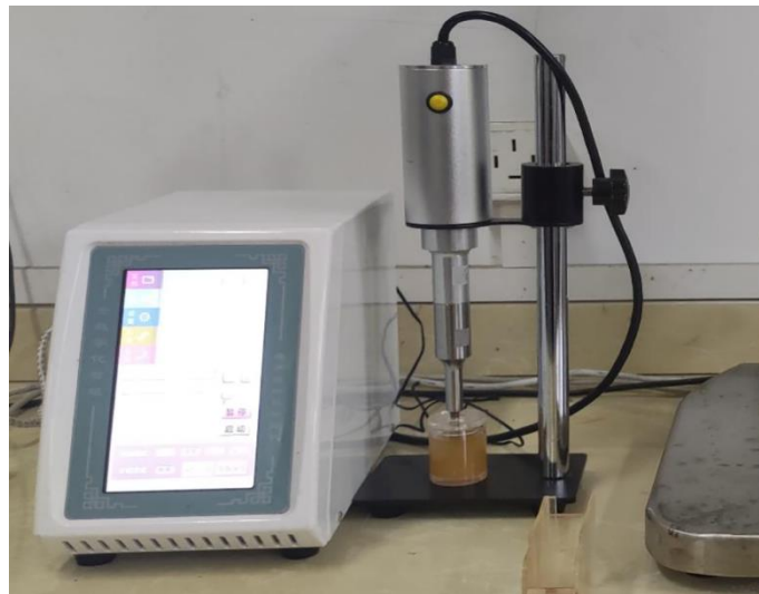
Fig. 2. Ultrasonic cell disruptor for ultrasonic treatment. (Fixed frequency: 20.056kHz,)
