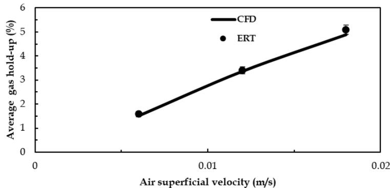
Fig. 3 (a). Comparison of sectional average gas holdup between CFD and ERT at different superficial air velocities
