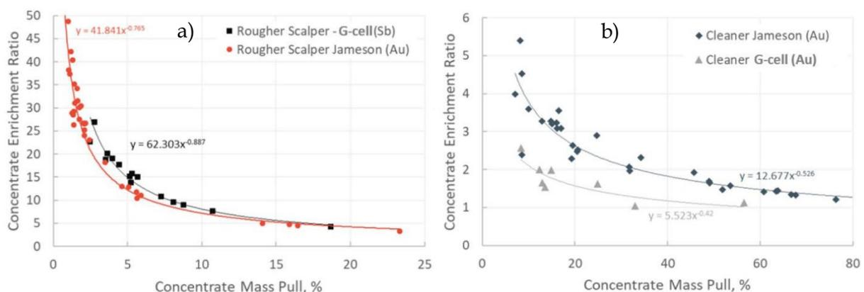
Fig. 9. Concentrate enrichment ratio vs. mass pull using both Imhoflot™ and Jameson™ cells at a) rougher scalper duty and b) cleaner stage (Pyle et al., 2022)
