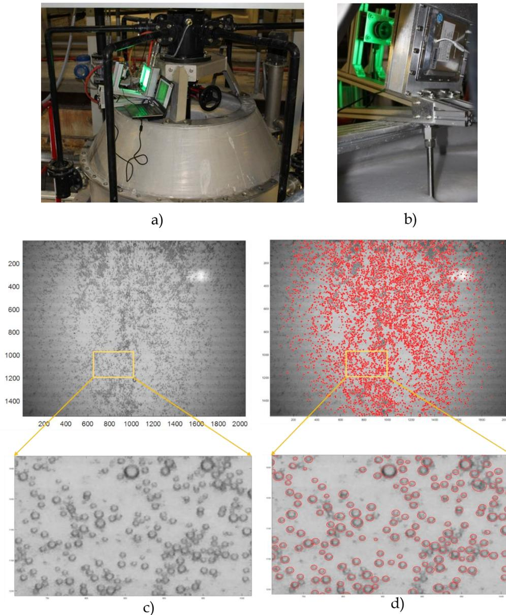
Fig. 4. a) Bubble viewer mounted on the Imhoflot™ H-16 (1.6 m diameter, 60 m<sup>3</sup>/h), b) sampling tube, viewing chamber and camera, c) original frame, and d) filtered image with analysed bubbles are marked with a circle
