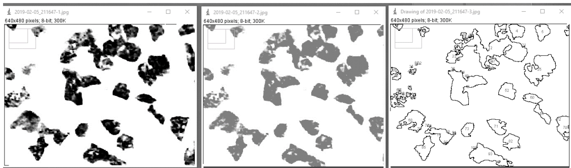
Fig. 2. The image processing steps in ImageJ software (1-Original; 2-Threshold; 3-Analyzed). The pattern of the quartz sample
