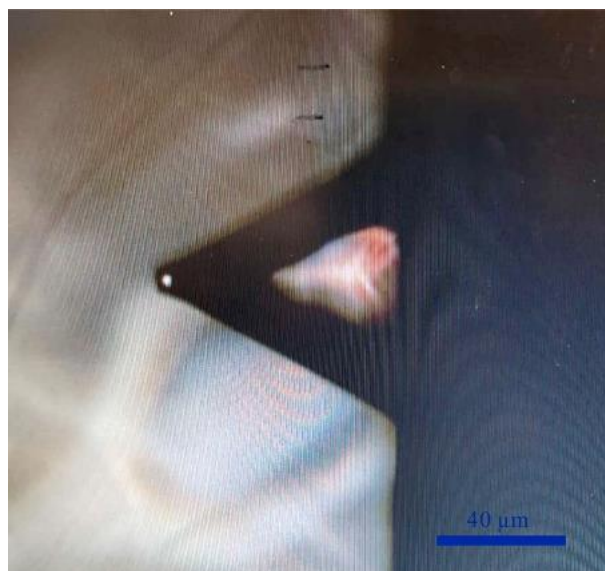
Fig. 2. Image of the hollow tip with the loading area partially filled with the glycerol/water mixture
