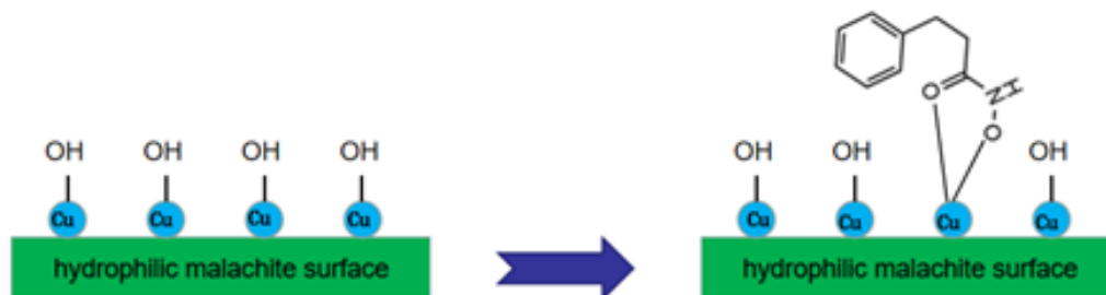
Fig. 12. Adsorption model of BPHA onto the surface of malachite
