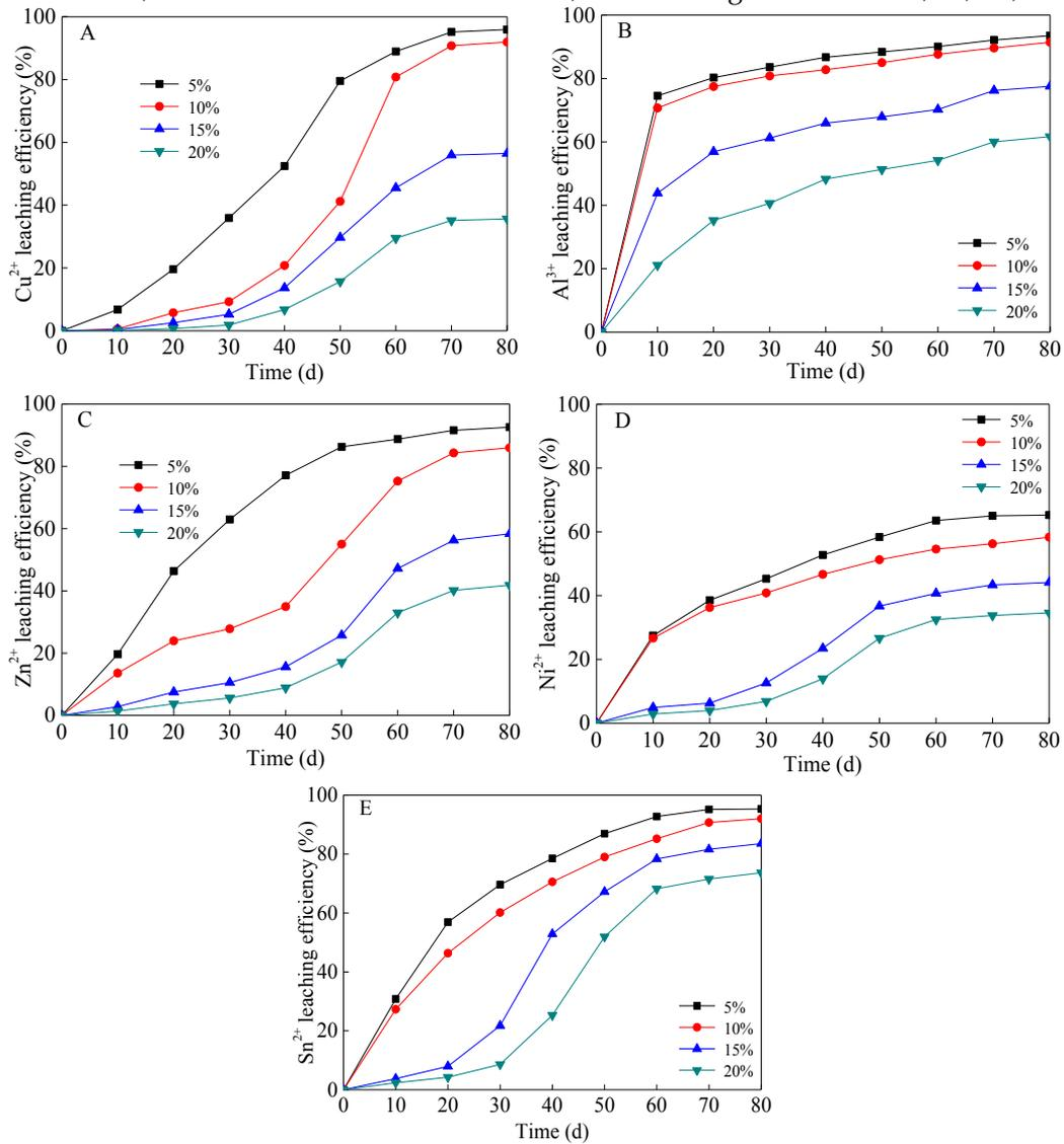
Fig. 5. Effect of WPCB concentration on Cu, Al, Zn, Ni, and Sn leaching efficiency (WPCB concentration of 5%, 10%, 15% and 20% (w/w))
