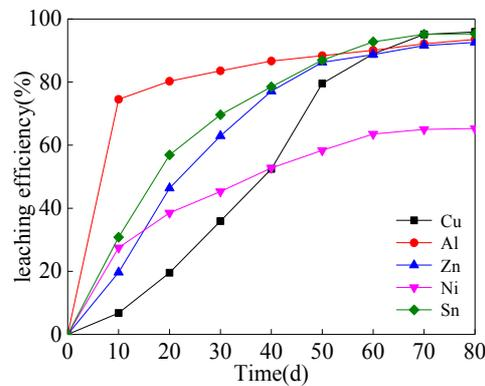
Fig. 9. Cu, Al, Zn, Ni, and Sn leaching efficiency under the optimal conditions
