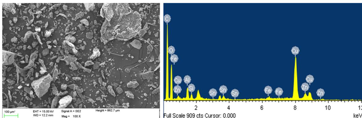
Fig. 1. SEM image and EDX analysis of WPCBs
