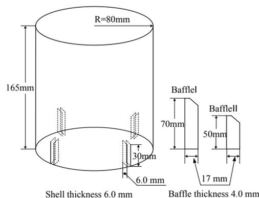
Fig. 3. Self-made stirred tank reactor
