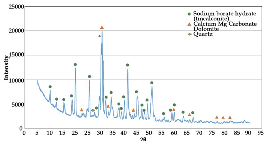
Fig. 4. The phase composition of the solid part of tailing
