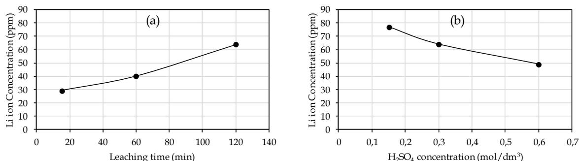
Fig. 11. a) A variation of Li-ion concentrations in PLS according to the leaching time, b) Effect of H<sub>2</sub>SO<sub>4</sub> concentrations on Li-ion concentration
