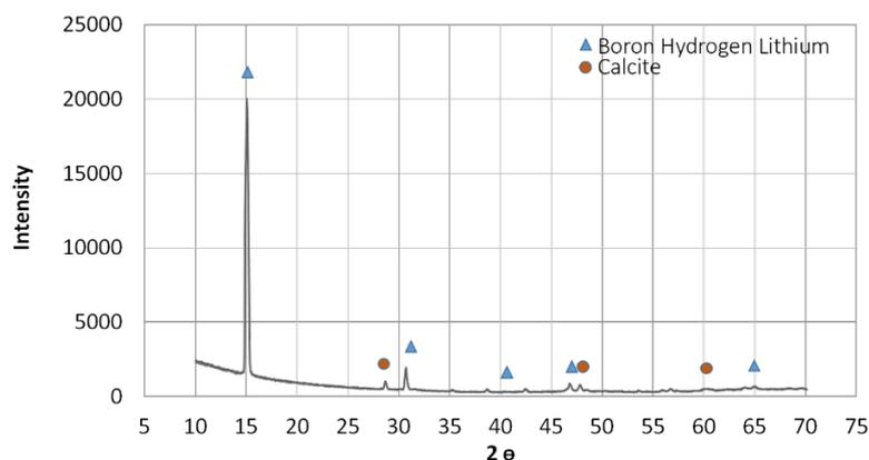
Fig. 9. The phase composition of the separated crystals
