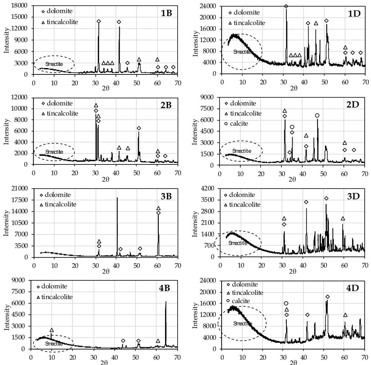
Fig. 6. The X-Ray diffraction pattern of solid samples
