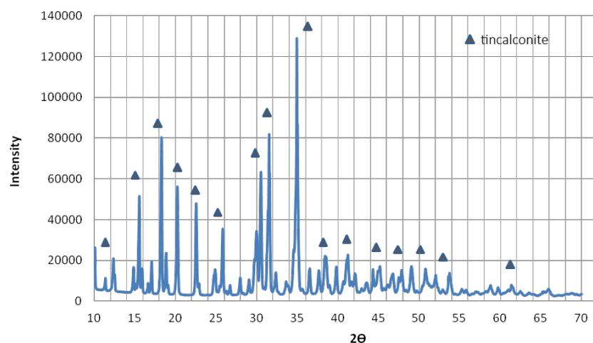
Fig. 10. The typical phase composition of glassy tinalconite
