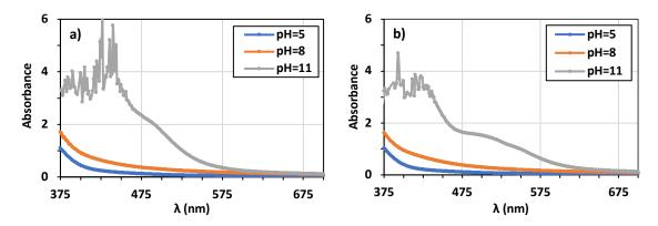
Fig. 4. UV-Vis spectra for samples synthesized at 35°C under aerobic conditions (a) and nitrogen atmosphere (b)
