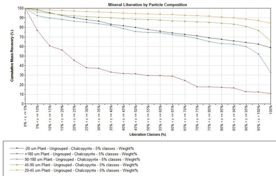
Fig. 8. Chalcopyrite mineral liberation by particle composition
