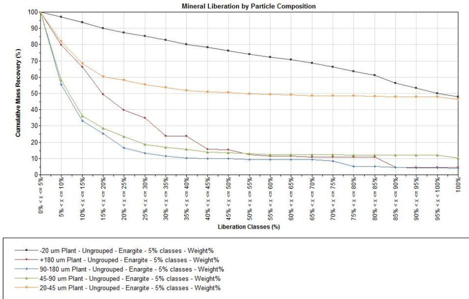
Fig. 9. Enargite/tennantite mineral liberation by particle composition
