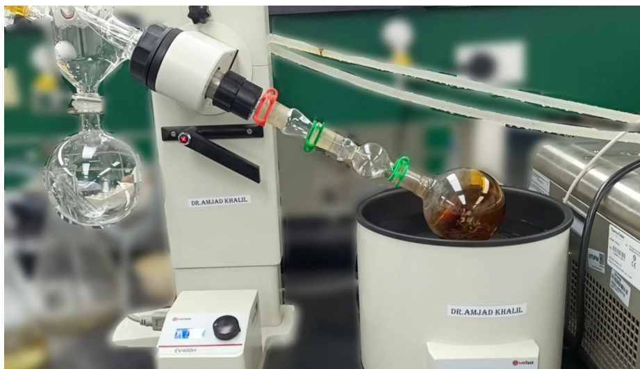
Figure 3. Sample drying in the rotary evaporator
