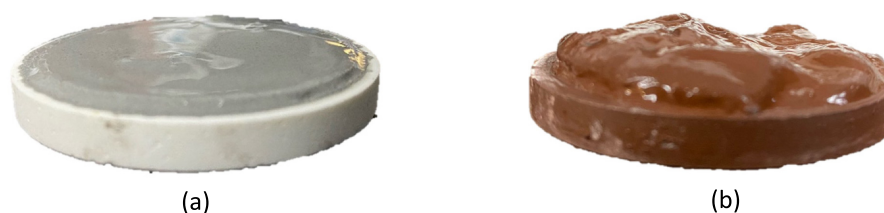
Figure 5. Sample filter cakes before removal: barite filter cake (a) and MicroMax filter cake (b)
