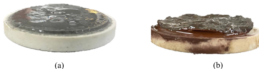
Figure 8. Filter cake after removal, Barite filter cake (a), MicroMax filter cake (b)
