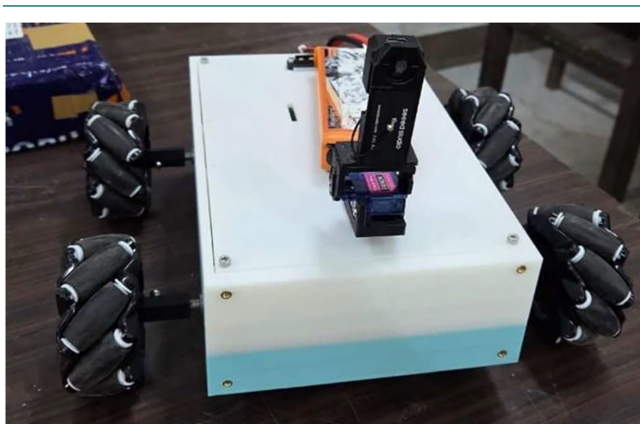
Figure 1. Top-down view of the assembled 4-wheel drive Mecanum robot platform showing the vision node, pan-tilt camera mount, and motor layout
