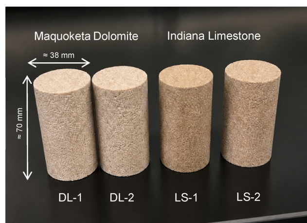
Figure 1. Geometry of core plugs used in this study
