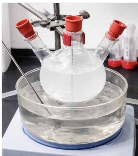
Figure 1. Drying setup with stirring and heating
