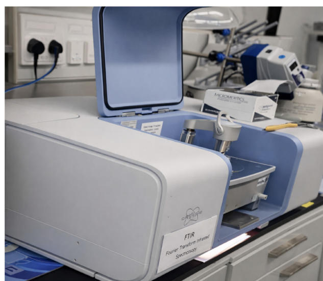
Figure 4. FTIR spectrometer used for functional group analysis
