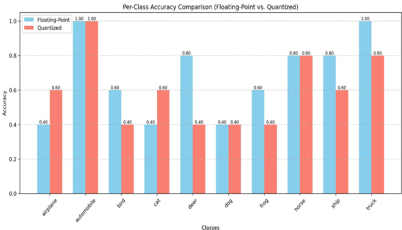
Figure 3. Accuracy comparison: FP32 vs. quantized model across CIFAR-10 classes
