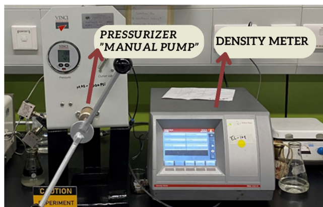
Figure 3. Density meter connected to a manual pump
