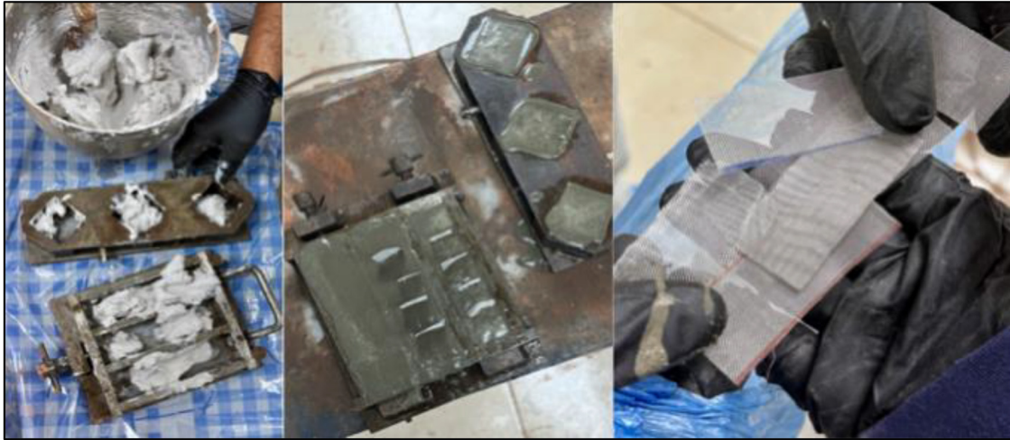
Figure 2. Casting of mortar specimens showing cubic and prismatic molds with metallic mesh electrodes embedded to enable electrical measurements
