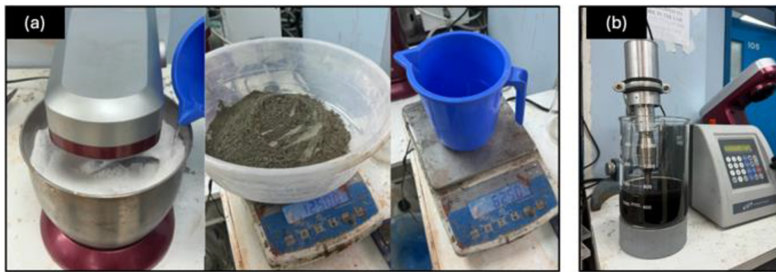
Figure 1. (a) Mixing and preparation of mortar specimens; (b) ultrasonication used to disperse GO in water before mixing
