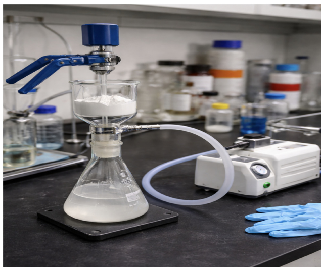
Figure 5. Vacuum filtration setup used for powder separation and collection
