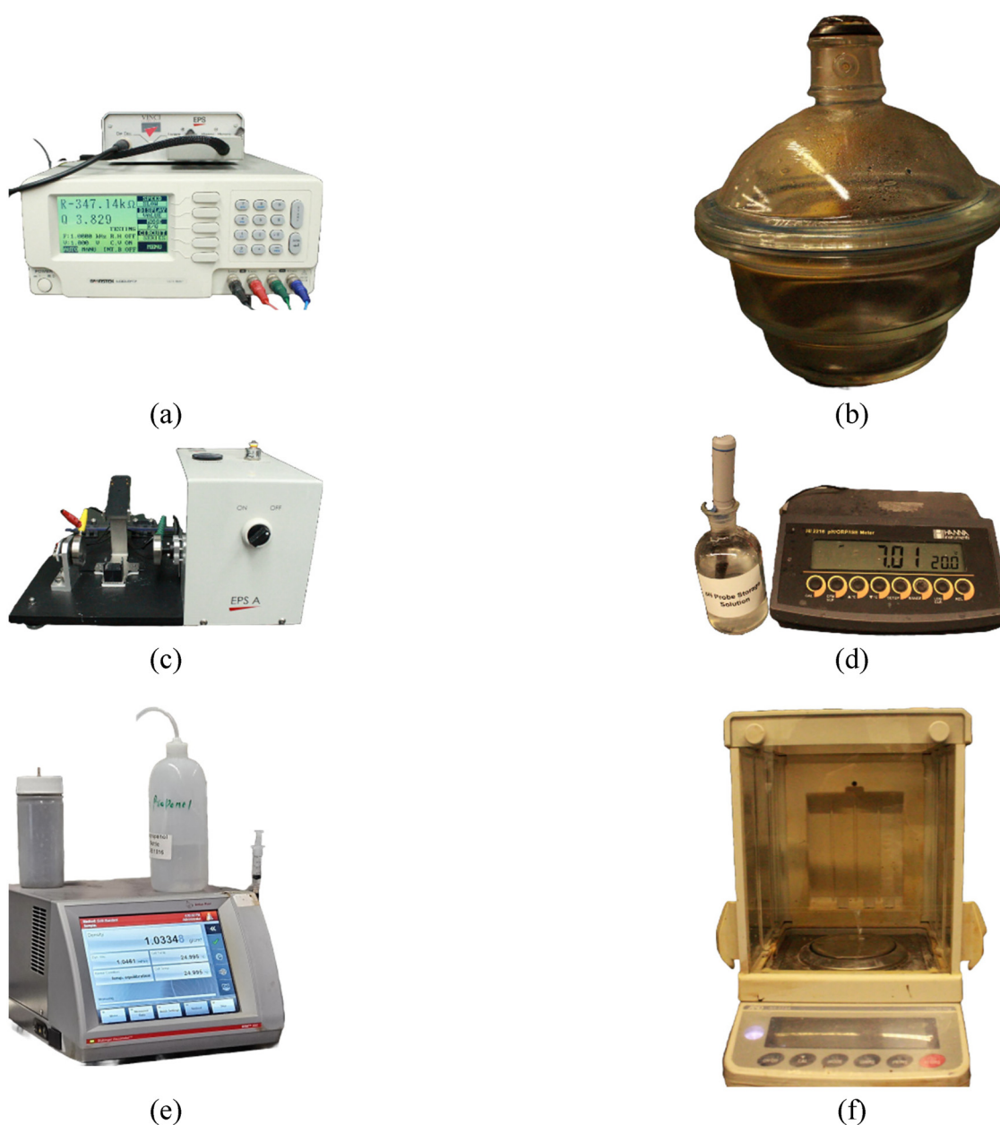
Figure 3. Experimental setup for carbonate brine characterization: (a) solution resistivity device; (b) vacuum saturation chamber for Austin Chalk cores; (c) GW Instek LCR 821 for resistivity measurements; (d) Hanna Instruments device for pH, redox potential, and temperature; (e) Anton Paar viscometer for viscosity and density; and (f) A&D GR semi-microbalance for solution preparation and porosity verification
