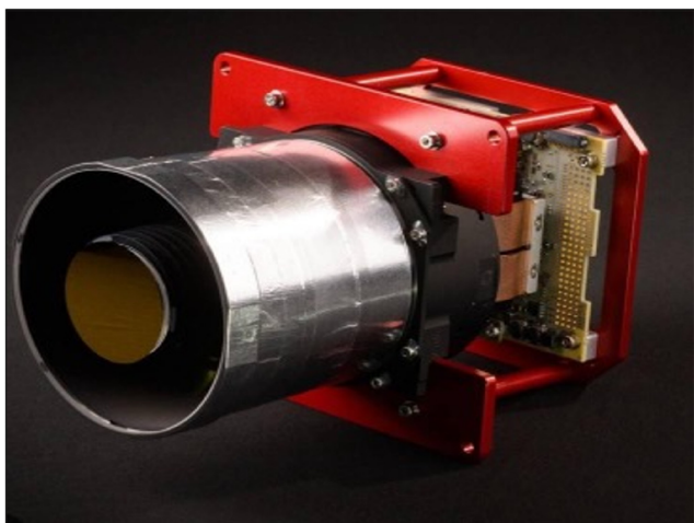
Figure 3. Representative CubeSat-class push broom optical payload used to illustrate typical Earth observation imaging configurations and mission simulation assumptions, based on the HyperScape100 hyperspectral imager 16
