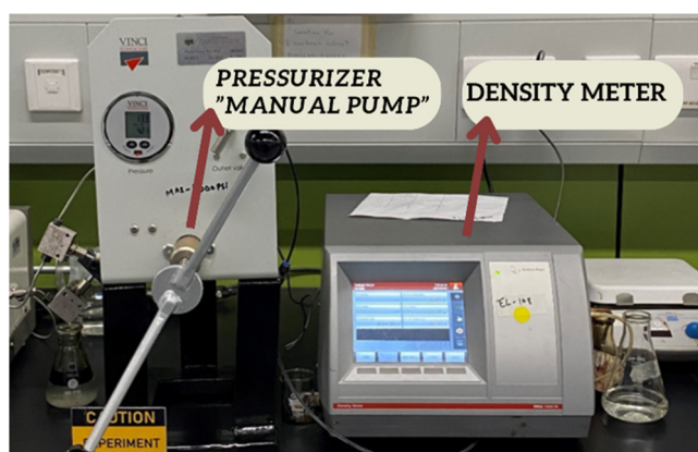
Figure 3. Density meter connected to a manual pump
