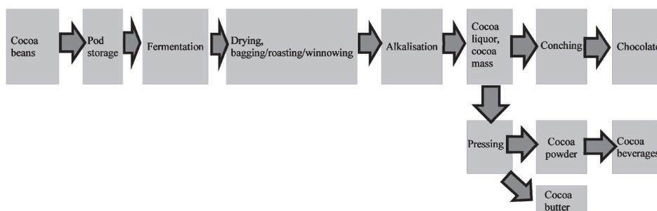
Fig. 1. The processing of cocoa beans (own elaboration)
