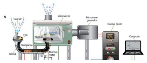
Fig. 2. Experimental set-up for drying processes: a – convective drying and infrared-assisted convective drying set-up; b – microwave-assisted convective drying set-up
