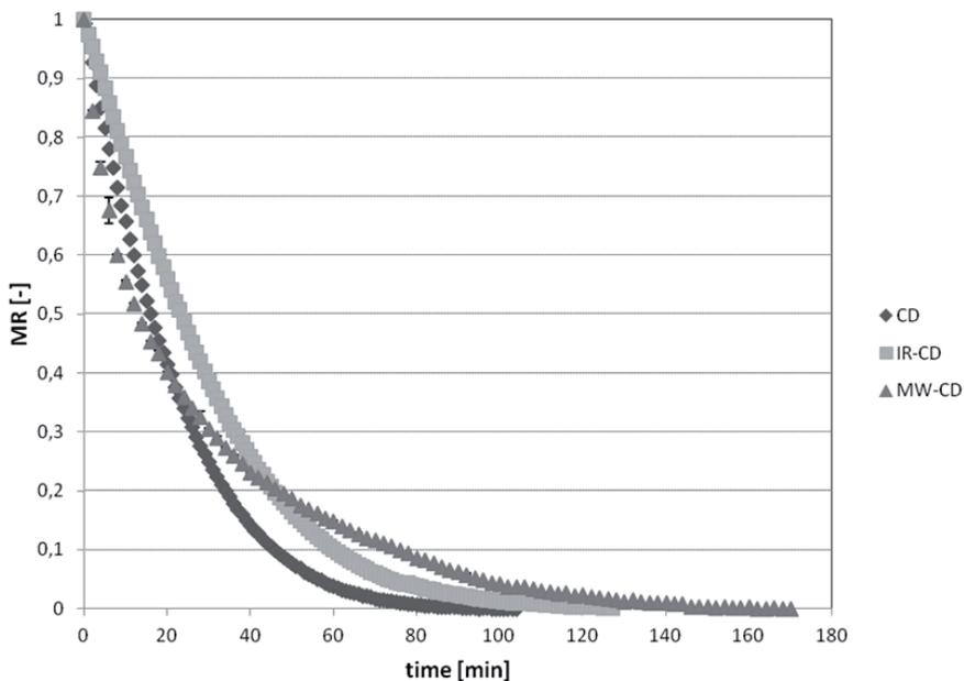
Fig. 3. The drying curves of radish sprouts dried by the different methods: CD – convective air-drying, IR-CD – infrared-assisted convective drying, MW-CD – microwave-assisted convective drying
