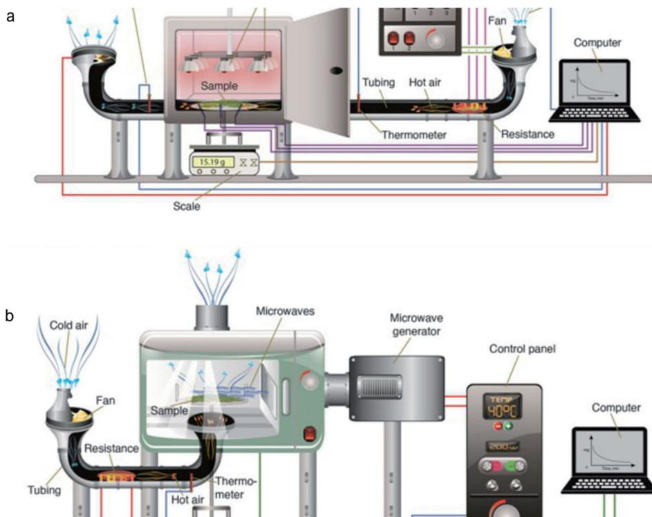
Fig. 2. Experimental set-up for drying processes: a – convective drying and infrared-assisted convective drying set-up; b – microwave-assisted convective drying set-up
