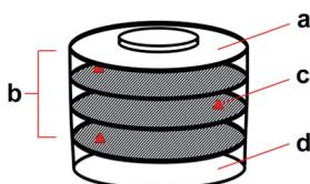
Fig. 1. Scheme of the sprouting vessel: a – lid; b – sprouting dishes with drainage channels; c – siphon; d – overflow tank
