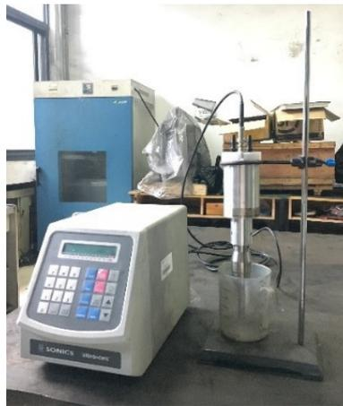
Fig. 2. Schematic of ultrasonic treatment experimental setup
