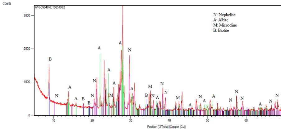
Fig. 1. XRD patterns of the nepheline syenite sample
