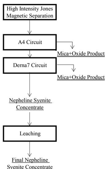
Fig. 10. Experiment flowsheet for magnetic separation and flotation followed by leaching
