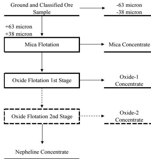
Fig. 4. General flowsheet for the flotation experiments
