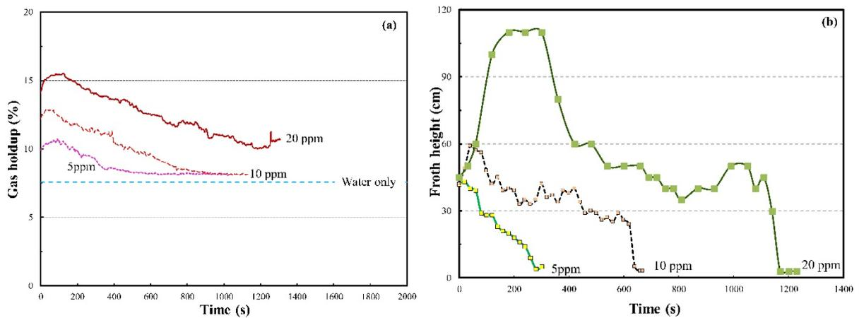
Fig. 2. Variation with time and concentration at natural pH: (a) Gas holdup; and (b) Froth height
