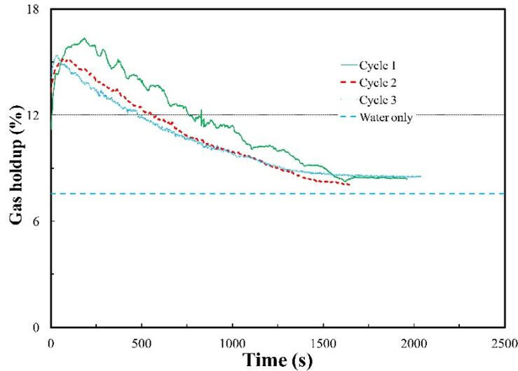
Fig. 4. Gas holdup as a function of time for three cycles
