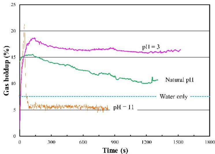
Fig. 5. Effect of pH on gas holdup as a function of time in 20 ppm DDA (including water only for reference)
