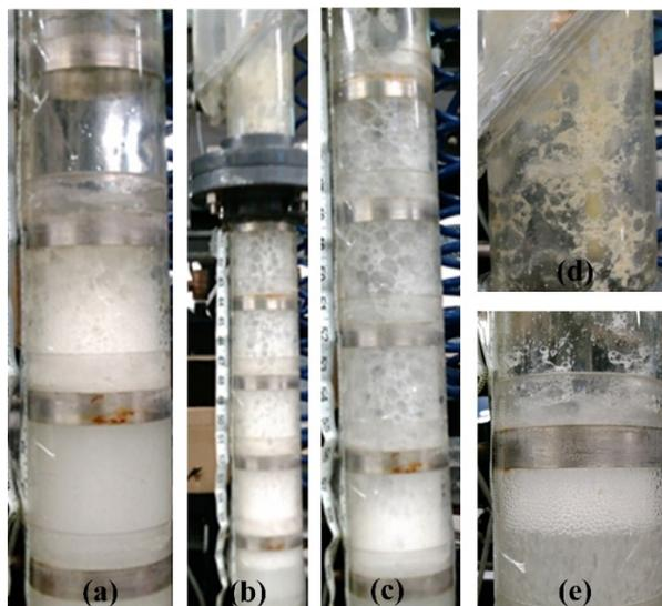
Fig. 3. Images of the froth with 20 ppm DDA at natural pH over time (view in conjunction with Fig 2(a)): (a) the start (i.e., on reaching  $J_g = 1.8\text{ cm/s}$ ); (b) 4 mins (240 s), close to max height; (c) 11 mins (660 s), significant decline in height with evidence of large bubbles; (d) yellow precipitates left on column wall; and (e) 18 mins (1080 s), froth virtually disappeared
