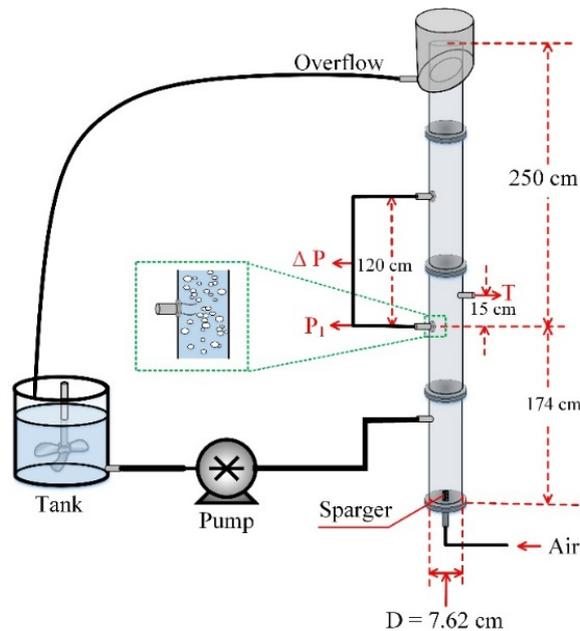
Fig. 1. Experimental setup to measure gas holdup and froth height
