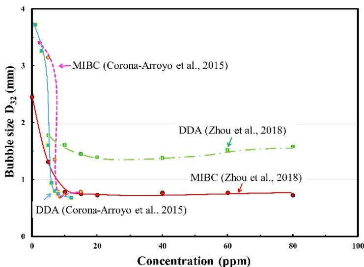
Fig. 6. Comparison of results for bubble size as a function of concentration for MIBC and DDA (data from Corona-Arroyo et al. (2015) and Zhou et al. (2018))
