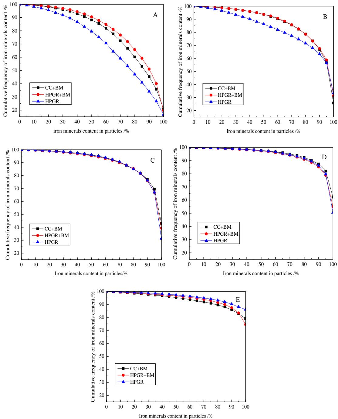
Fig. 9. Degree of liberation curves for iron minerals in the grinding products: A)  $+0.100$  mm size fraction; B)  $-0.100+0.074$  mm size fraction; C)  $-0.074+0.043$  mm size fraction; D)  $-0.043+0.031$  mm size fraction; E)  $-0.031+0.015$  mm size fraction
