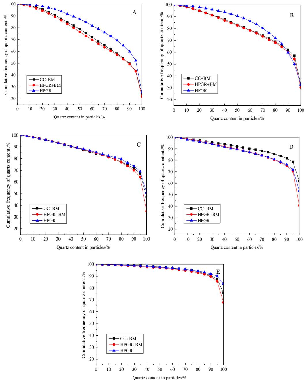
Fig. 8. Degree of liberation curves for quartz in the grinding products: A) +0.100 mm size fraction; B) - 0.100+0.074 mm size fraction; C) -0.074+0.043 mm size fraction; D) -0.043+0.031 mm size fraction; E) - 0.031+0.015 mm size fraction
