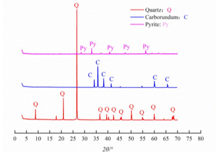
Fig. 2. X-ray diffraction spectrograms of pure minerals
