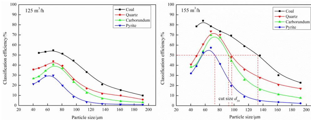
Fig. 6. Actual classification efficiency curves
