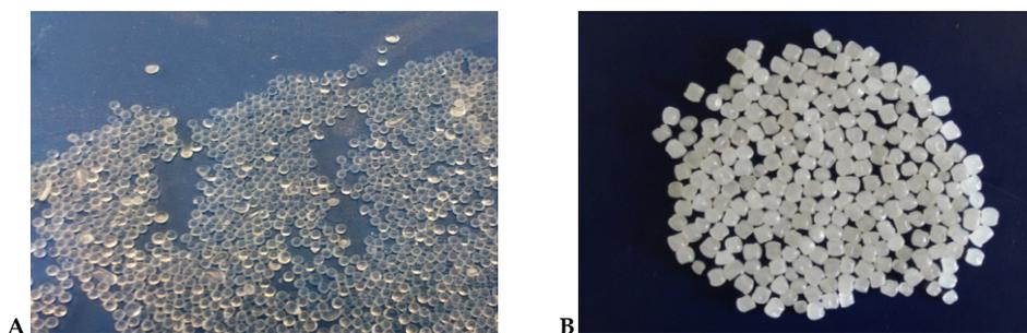
Fig. 2. (A) Glass beads, (B) Polyethylene pellets
