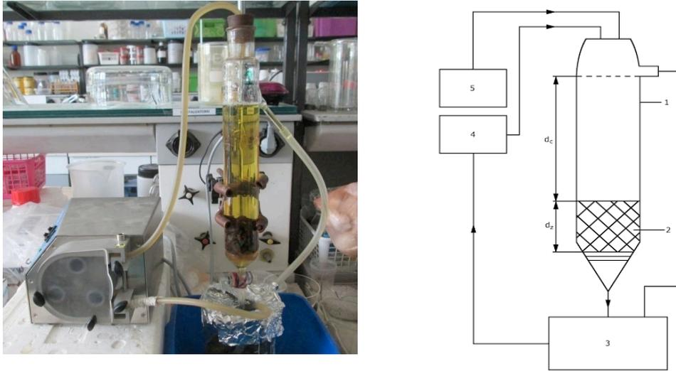
Fig. 3. Bioleaching column: 1 - bioreactor, 2 - bed, 3 - container with leaching solution, 4 - peristaltic pump, 5 - air pump
