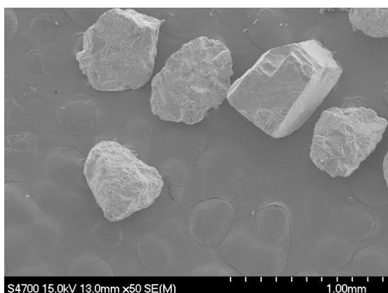
**Fig. 2.** SEM picture of dolomite particles (- 0.40 + 0.50 mm).
