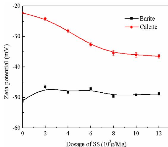
Fig. 8. Zeta potentials of barite and calcite versus SS dosage with SDS  $2 \cdot 10^3$  g/Mg at pH 9.0
