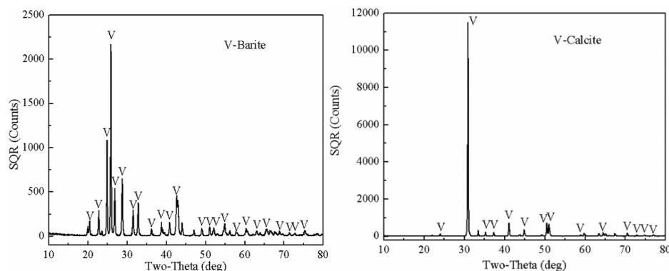
Fig. 1. XRD diagrams of barite and calcite
