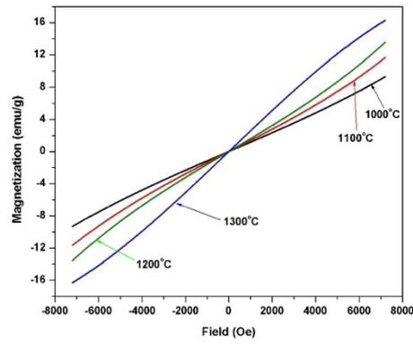
Fig. 6. Effect of calcination temperature on the M-F hysteresis loop of  $\text{Fe}_2\text{TiO}_5$  synthesized at pH 9.1
