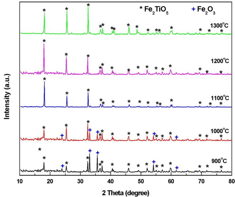
Fig. 2. XRD patterns of the produced  $\text{Fe}_2\text{TiO}_5$  at pH 9.1
