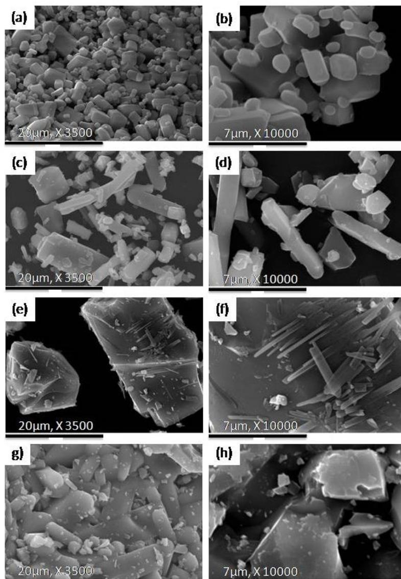
Fig. 4. SEM micrograph of the produced nanocrystalline  $\text{Fe}_2\text{TiO}_5$  powders from the ilmenite ore at pH 9.1 and calcined at (a, b) 1000 °C, (c, d) 1100 °C, (e, f) 1200 °C, and (g, h) 1300 °C
