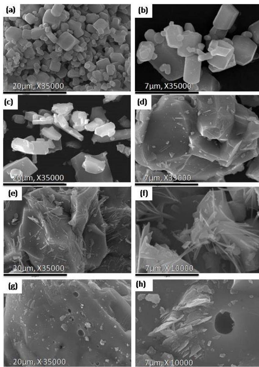
Fig. 5. SEM micrograph of the produced nanocrystalline  $\text{Fe}_2\text{TiO}_5$  powders from the ilmenite ore at pH 11.2 and calcined at; (a, b) 1000 °C, (c, d) 1100 °C, (e, f) 1200 °C, and (g, h) 1300 °C
