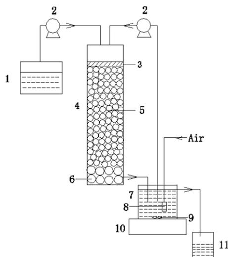
Fig. 1. Schematic of the column reactor system: 1- glass container serving as the culture medium reservoir; 2- peristaltic pump; 3- gauze; 4- column; 5- mid-low grade PR; 6- support gravel; 7- plastic container serving as an internal recirculation reservoir; 8- aerator connected to compressed air tank; 9- mixer; 10- magnetic stirring plate; 11- disposal bottle
