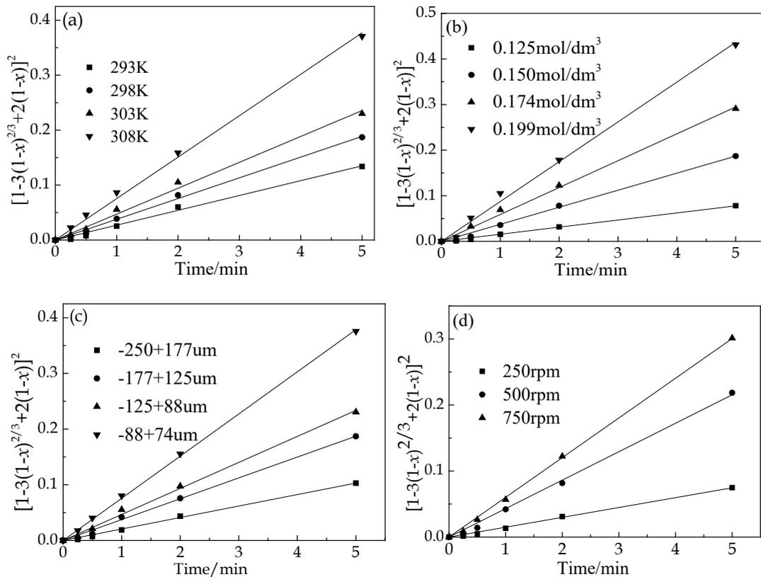
Fig. 3. Plot of  $[1-3(1-x)^{2/3}+2(1-x)]^2$  vs. time for different operation parameters: (a) temperature, (b) MSA concentration, (c) particle size, and (d) stirring speed
