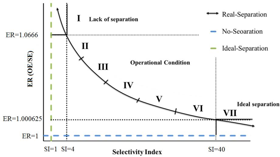
Fig. 6. New upgrading curve based on efficiency ratio (ER) as a function of selectivity index (SI)
