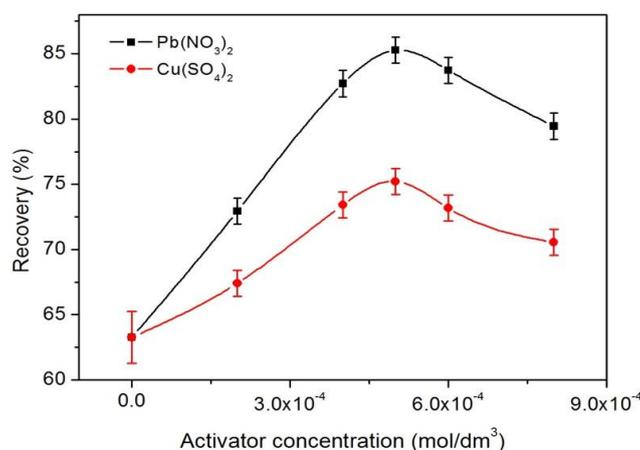
Fig. 2. Effect of activators concentration on stibnite flotation (concentration of BX is  $1 \times 10^{-5}$  mol/dm<sup>3</sup> and the pH is 6.5)
