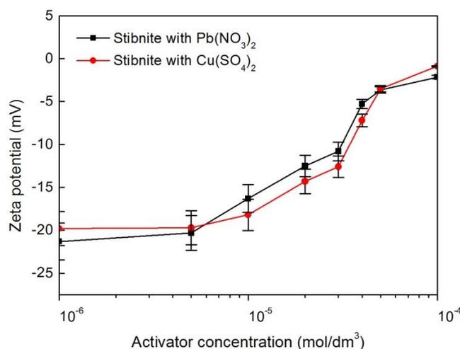
Fig. 3. Effect of  $\text{CuSO}_4$  and  $\text{Pb}(\text{NO}_3)_2$  concentration on zeta potential of stibnite at the pH of 6.5
