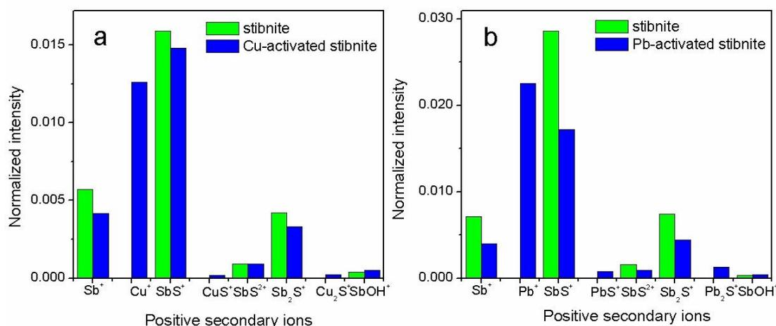
Fig. 5. Positive secondary ions spectra of natural stibnite and stibnite treated with  $5 \times 10^{-5}$  mol/dm<sup>3</sup>  $\text{CuSO}_4$  (a) and  $\text{Pb}(\text{NO}_3)_2$  (b)
