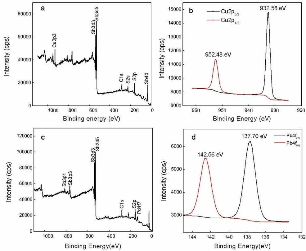
Fig. 4. XPS spectra for the stibnite surface treated with  $5 \times 10^{-5}$  mol/dm<sup>3</sup>  $\text{CuSO}_4$  (a, b) and  $5 \times 10^{-5}$  mol/dm<sup>3</sup>  $\text{Pb}(\text{NO}_3)_2$  (c, d)
