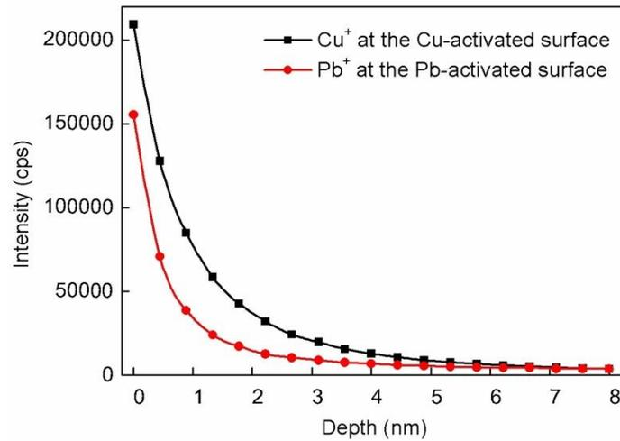
Fig. 7. Depth profiles of characteristic secondary ions in the positive mode for the stibnite treated with  $5 \times 10^{-5}$  mol/dm<sup>3</sup> of  $\text{CuSO}_4$  or  $\text{Pb}(\text{NO}_3)_2$
