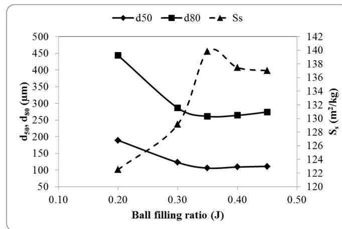
Fig. 4. The results of ball filling ratio tests
