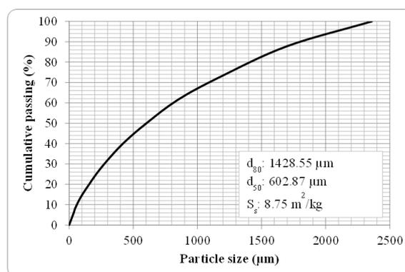
Fig. 1. The size distribution of the feed material
