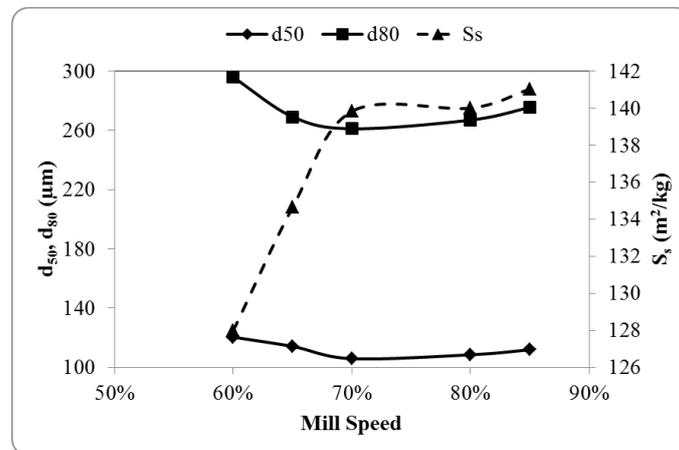
Fig. 3. The results of mill speed tests
