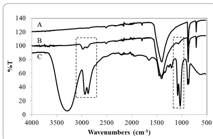
Fig. 10. FTIR spectra of no aid condition (A), product (B) and commercial liquid grinding aid (C)
