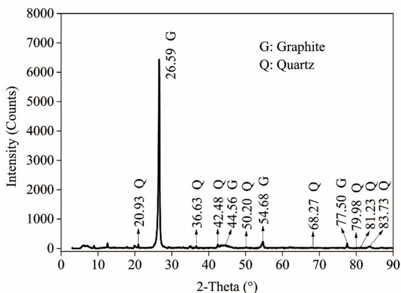
Fig. 1. XRD patterns of the graphite ore
