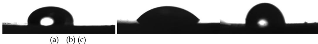
Fig. 14. Contact angles of calcium stearate (a), unmodified calcite (b) and modified calcite (c)
