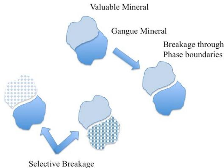
Fig. 1. Schematic representation of breakage patterns of mineral particles
