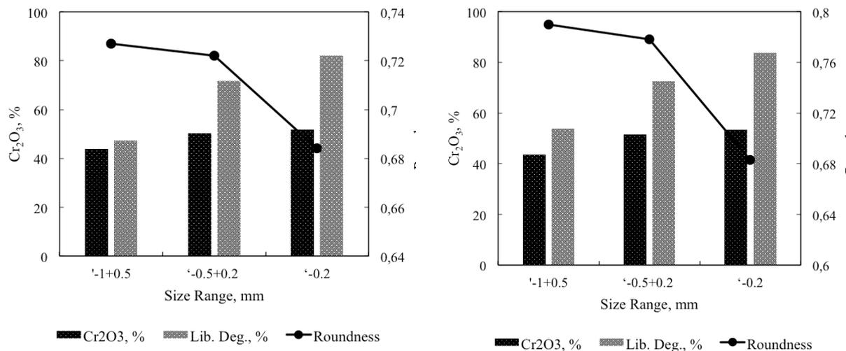
Fig. 4. The effects of different breakage mechanisms on liberation degree, roundness and metal recovery values of concentrates, (Left: Compression Breakage, Right: Impact Breakage)
