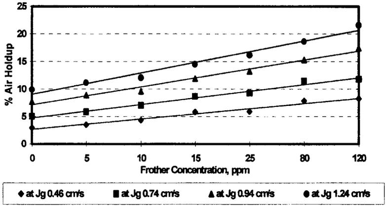
Fig. 3. Effect of frother concentration on air holdup at different superficial air velocity
