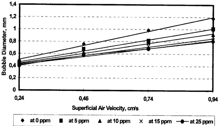
Fig. 2. Effect of superficial air velocity on air bubble diameter
