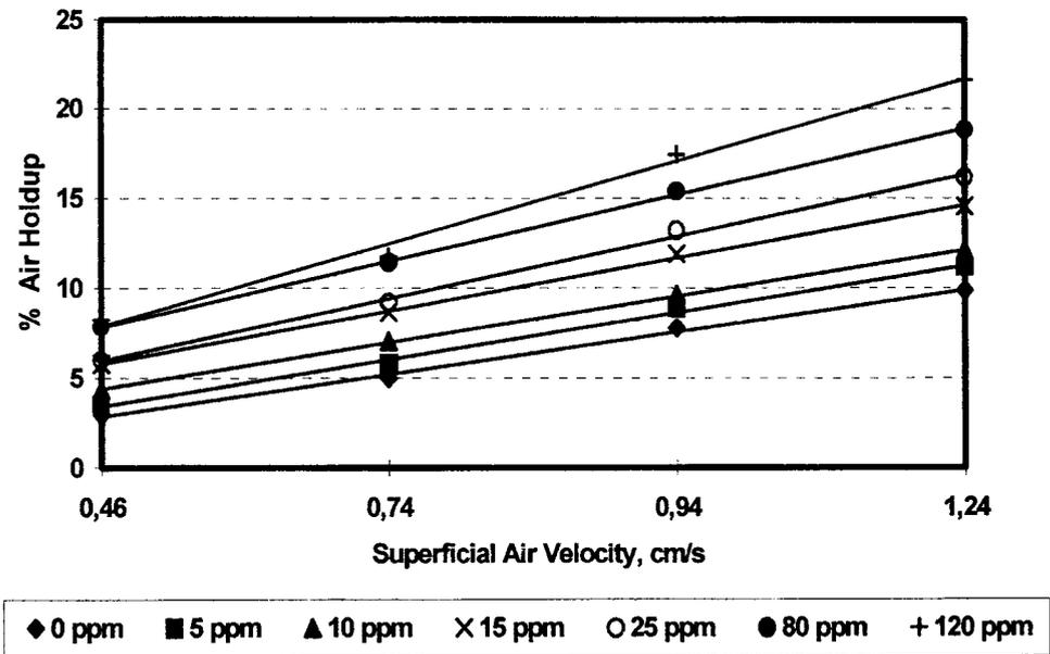
Fig. 1. Effect of superficial air velocity on air holdup at different frother dosages
