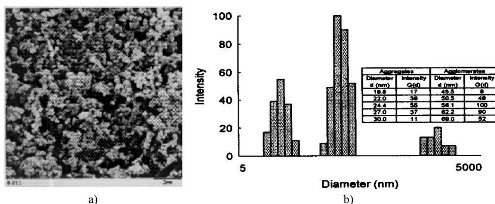
Fig. 1.a) SEM and b) particle size distribution of unmodified TiO<sub>2</sub>
