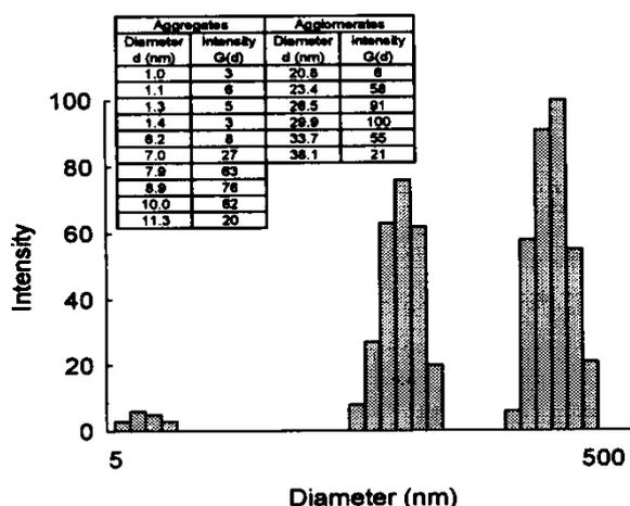
Fig. 4. Particle size distribution of  $\text{TiO}_2$  modified with U-15D silane
