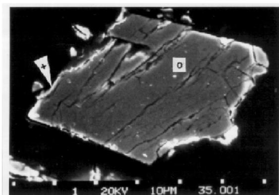
Fig. 2. SEM photograph of millerite particle cross-section after 5 hours leaching in 0.2M  $\text{Fe}_2(\text{SO}_4)_3$  – 1.0M  $\text{H}_2\text{SO}_4$  solution at 95°C; two different phases – grey and white – are denoted by o and +, respectively.
