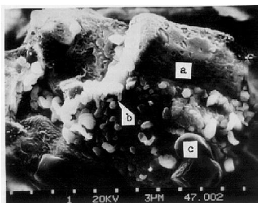
Fig. 1. SEM photograph of millerite leach residue after 5 hours leaching in 0.2M FeCl<sub>3</sub> - 0.2M CuCl<sub>2</sub> - 1.0M HCl - 2.0M NaCl solution at 95°C; (a) - leached millerite, (b) - small sulphur granules, (c) - large sulphur granules
