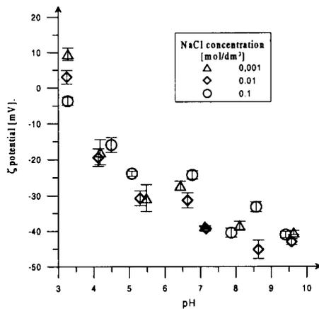
Fig. 12. Zeta potential as a function of pH and electrolyte concentration for the  $\text{Mn}_2\text{O}_3/\text{NaCl}$  solution system
