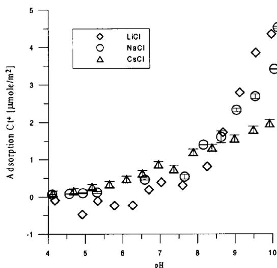
Fig 7. Adsorption of cations ( $C_t = \text{Li}, \text{Na}, \text{Cs}$ ) vs pH at the  $\text{MnO}_2/0,001 \text{ M. CtCl}$  electrolyte interface
