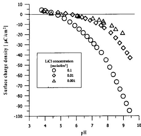
Fig. 1. Surface charge density as a function of pH and electrolyte concentration for the  $MnO_2/LiCl$  solution system
