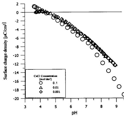
Fig. 3. Surface charge density as a function of pH and electrolyte concentration for the  $\text{MnO}_2/\text{CsCl}$  solution system
