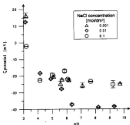
Fig. 5. Zeta potential as a function of  $\text{pH}$  and electrolyte concentration for the  $\text{MnO}_2/\text{NaCl}$  solution system
