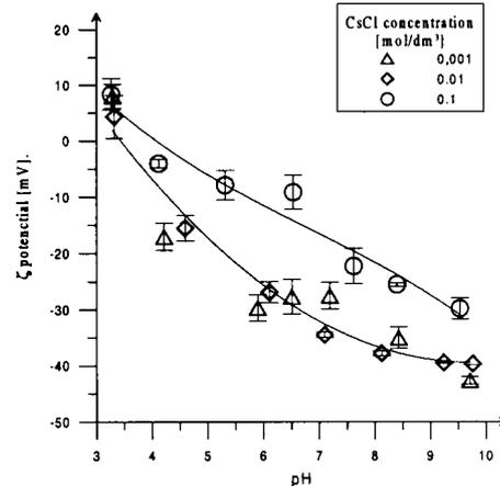
Fig. 13. Zeta potential as a function of pH and electrolyte concentration for the  $\text{Mn}_2\text{O}_3/\text{CsCl}$  solution system
