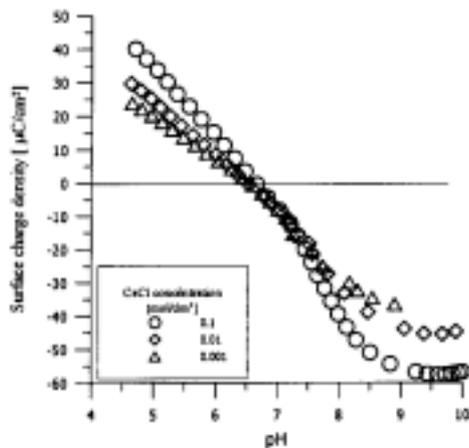
Fig. 10. Surface charge density as a function of pH and electrolyte concentration for the  $\text{Mn}_2\text{O}_3/\text{CsCl}$  solution system
