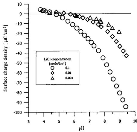
Fig. 1. Surface charge density as a function of pH and electrolyte concentration for the  $\text{MnO}_2/\text{LiCl}$  solution system
