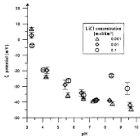
Fig. 11. Zeta potential as a function of pH and electrolyte concentration for the  $\text{Mn}_2\text{O}_3/\text{LiCl}$  solution system
