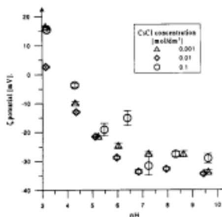
Fig. 6. Zeta potential as a function of  $\text{pH}$  and electrolyte concentration for the  $\text{MnO}_2/\text{CsCl}$  solution system.
