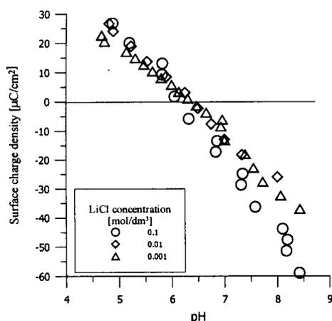
Fig. 8. Surface charge density as a function of pH and electrolyte concentration for the  $\text{Mn}_2\text{O}_3$ /LiCl solution system
