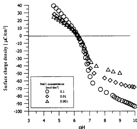
Fig. 9. Surface charge density as a function of pH and electrolyte concentration for the  $\text{Mn}_2\text{O}_3$ /NaCl solution system
