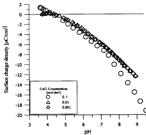
Fig. 3. Surface charge density as a function of pH and electrolyte concentration for the  $MnO_2/CsCl$  solution system
