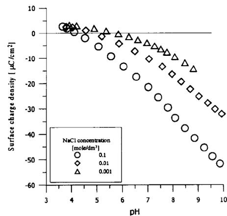
Fig. 2. Surface charge density as a function of pH and electrolyte concentration for the  $MnO_2/NaCl$  solution system
