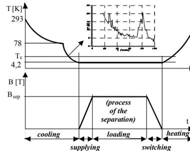
Fig. 11. Operation cycle of superconductor separator (Cieśla, 2003)
