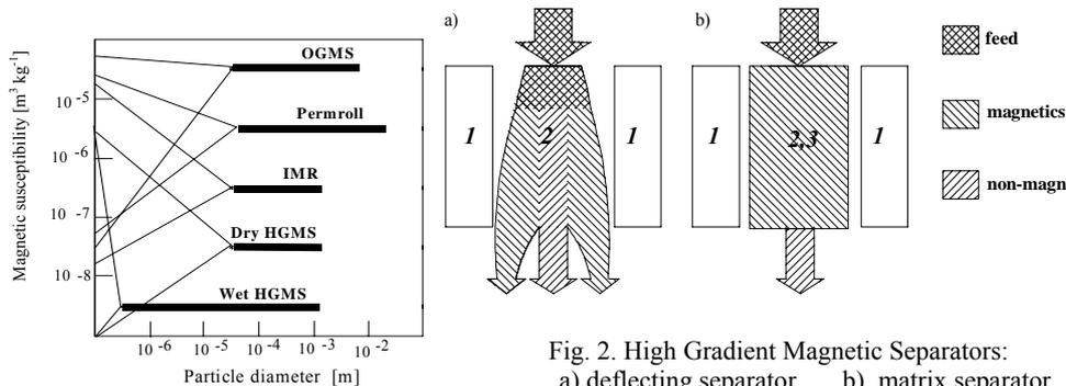
Fig. 2. High Gradient Magnetic Separators:
