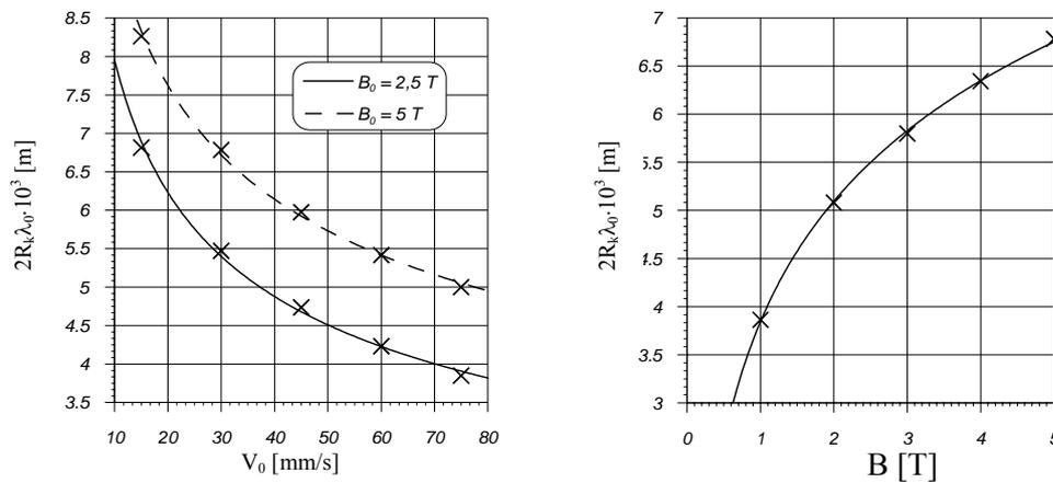
Fig. 5. “Pick up” zone width ( $2R_k\lambda_0$ ) vs. velocity of slurry flow through the matrix separator for induction  $B_0 = 2,5$  T and  $B_0 = 5$  T (a) and magnetic field induction in separator matrix for  $v_0 = 0.03$  ms $^{-1}$  (b) (Cieřla, 2000)
