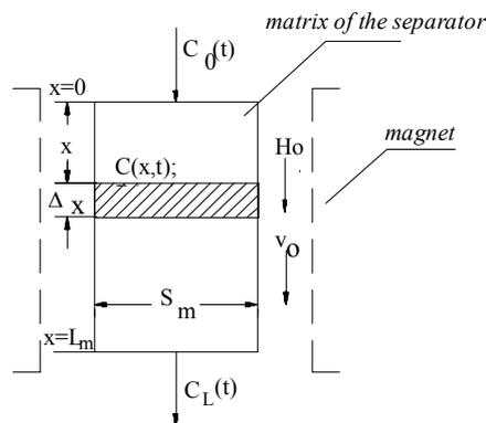
Fig. 3. Slurry of concentration  $C_0(t)$  is flowing across the matrix separator (Cieřla, 1996)
