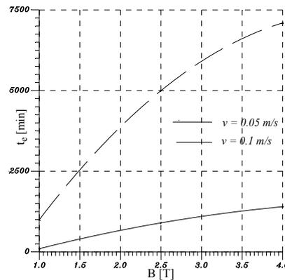
Fig. 7. Effective filtration time  $t_e$  vs. magnetic induction  $B$  (Cieśla, 2000)
