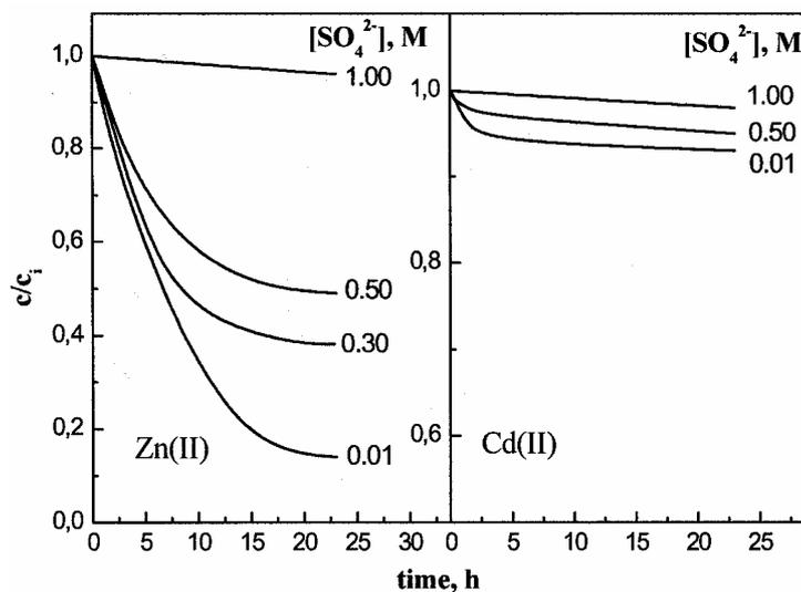
Fig. 3. Kinetics of zinc(II) and cadmium(II) transport through PIM with D2EHPA from source aqueous phase vs.  $\text{Na}_2\text{SO}_4$  concentrations, ( $c_{\text{Me}} = 1.0 \cdot 10^{-2}$  M), pH = 4.0. Membrane:  $2.6 \text{ cm}^3$  ONPOE / 1g CTA, 1.5 M D2EHPA
