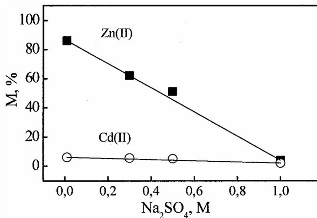
Fig. 4. Percent removal of zinc(II) and cadmium(II) ions through PIM from source aqueous phase containing equimolar mixture of both metals ( $c_{\text{Me}} = 1.0 \cdot 10^{-2}$  M) vs.  $\text{Na}_2\text{SO}_4$  concentration in source phase. Experimental conditions as in Fig.3
