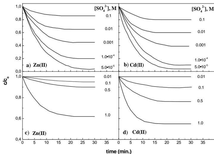
Fig. 1. Rate curves of zinc(II) and cadmium(II) concentration vs. time from aqueous solution containing equimolar mixture of both metals ( $c_{Me} = 1.0 \cdot 10^{-5} \text{ M}$ ) in presence of sulfates with DBSNa (a, b) and with CPCl (c, b),  $c_{surf.} = 2.0 \cdot 10^{-4} \text{ M}$
