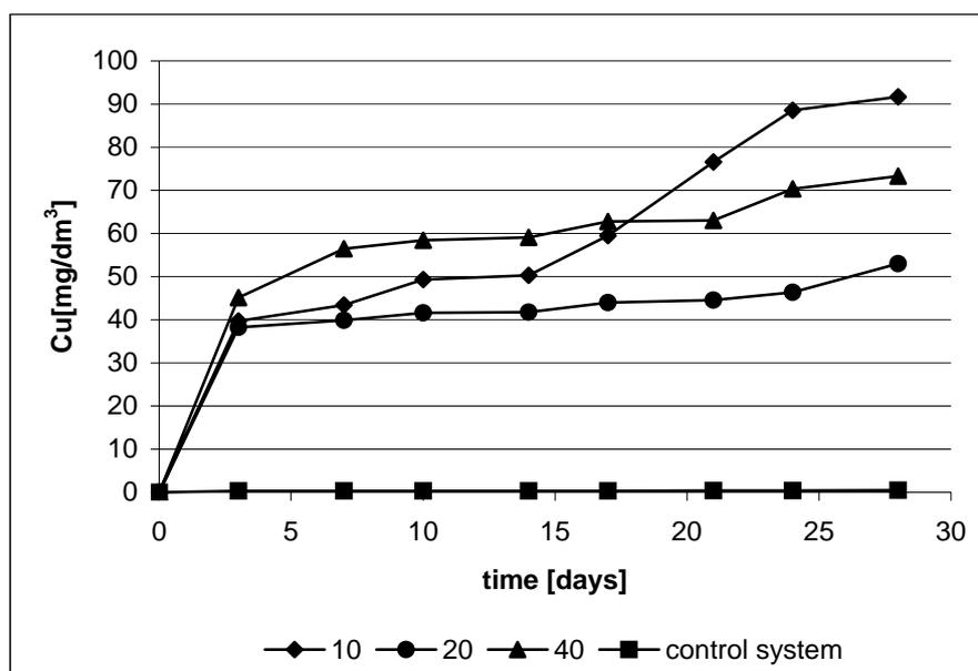
Fig. 1. The effect of temperature on the copper bioleaching during 28 days of process (10°, 20° and 40°C)
