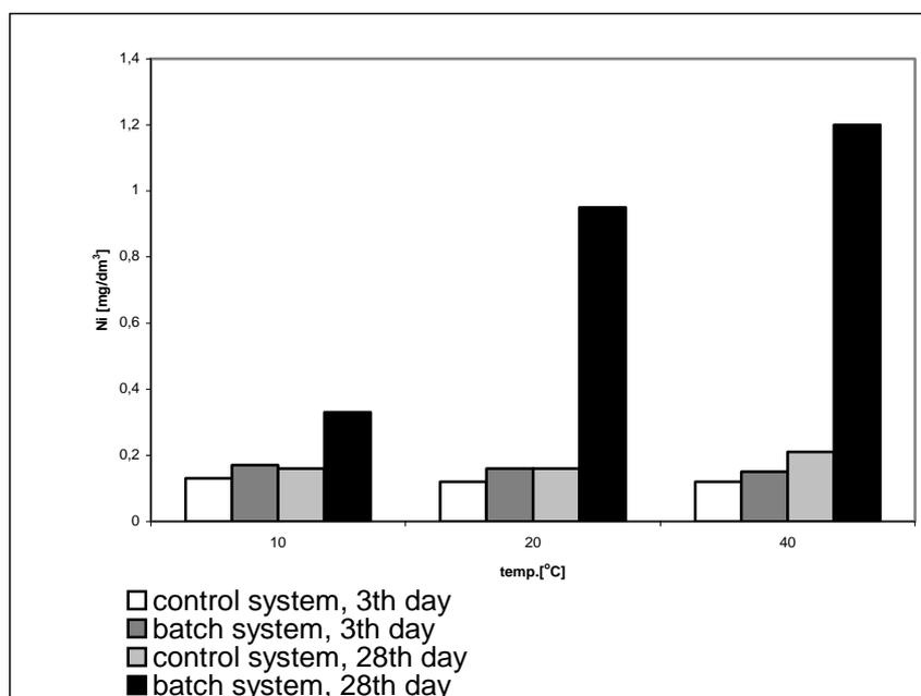
Fig. 2. The effect of temperature on Ni bioleaching during 28 days of process
