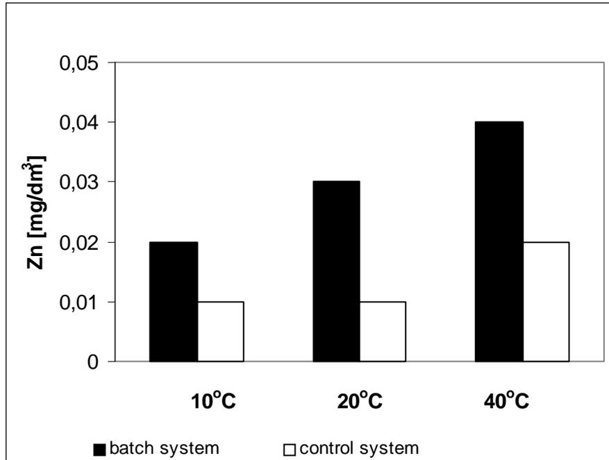
Fig. 3. The bioleaching of Zn during 28 days of process at 10°, 20° and 40 °C
