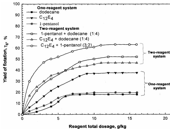
Fig. 1. Effect of one reagent and two-reagent dosage on flotation yield of coal using normal flotation procedure
