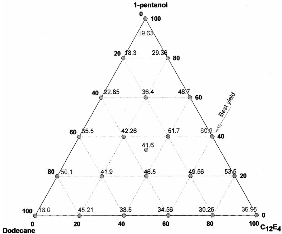
Fig. 2. Effect of dodecane - C<sub>12</sub>E<sub>4</sub> - 1-pentanol combinations on clean coal yield, at a total dosage of 10 g/kg using normal flotation procedure. Ratios among the three reagents are the same as read from ternary plot. Circles represent studied points, numbers show clean coal yield
