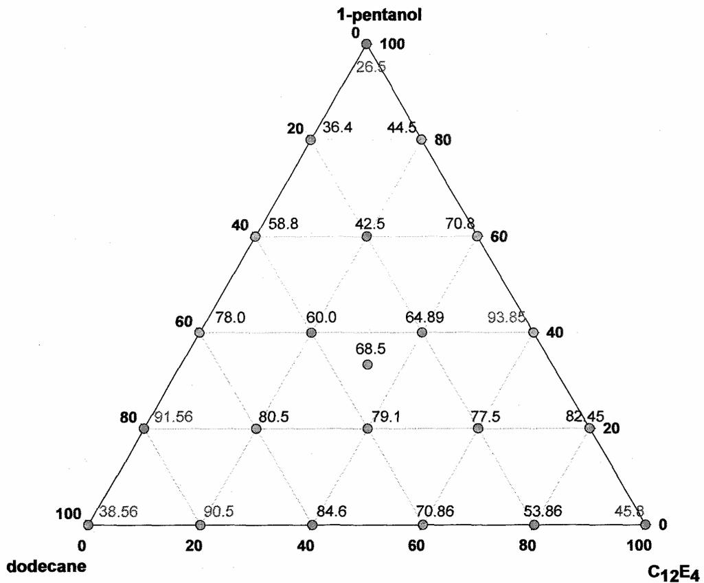
Fig. 6. Effect of dodecane -  $C_{12}E_4$  - 1-pentanol combinations on clean coal yield, at a total dosage of 16 g/kg using direct contact flotation procedure. Ratios (in wt. %) among the three reagents are the same as read from ternary plot. Circles represent studied points, numbers show clean coal yield
