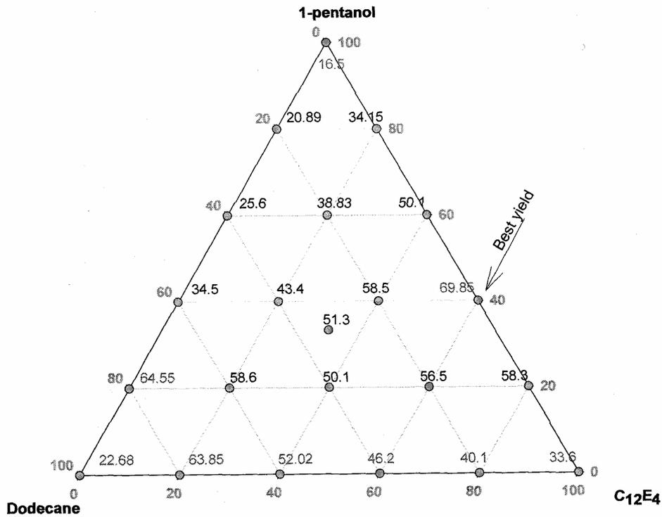
Fig. 5. Effect of dodecane - C<sub>12</sub>E<sub>4</sub> - 1-pentanol combinations on clean coal yield, at a total dosage of 8 g/kg using direct contact flotation procedure. Ratios (in wt. %) among the three reagents are the same as read from ternary plot. Circles represent studied points, numbers show clean coal yield
