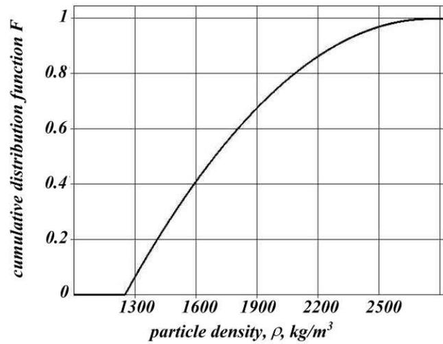
Fig. 2. Cumulative distribution function of particle density
